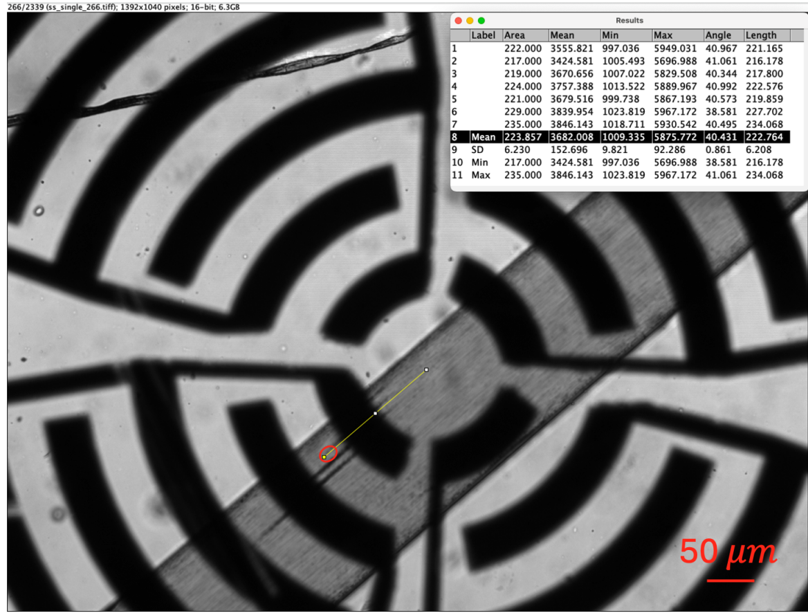
Figure 3.11: Measurement of the distance of the particle cluster's trajectory using ImageJ's line tool (yellow). The red circle highlights the cluster's end position.
