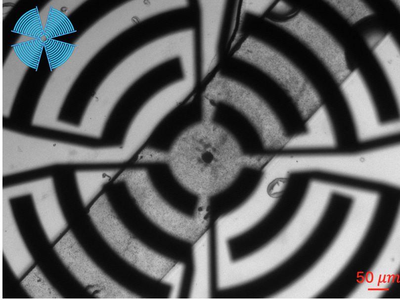
Figure 4.1: FIDT manipulating/capturing PS particles at a resonance frequency of 39.2 MHz, in a channel with a width of 300 \mu\text{m} and a height of 240 \mu\text{m}
